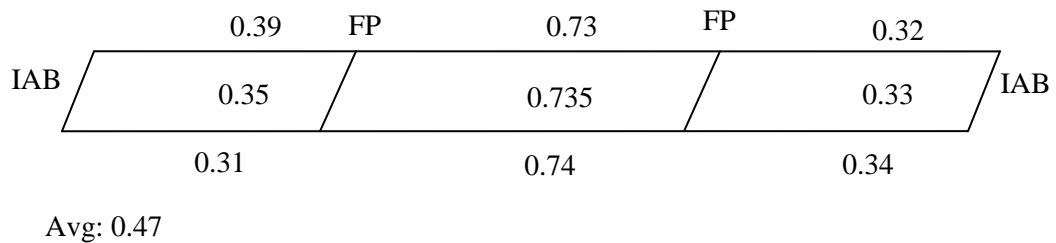
Figure 6.65. Change in length per span Bridge 109
