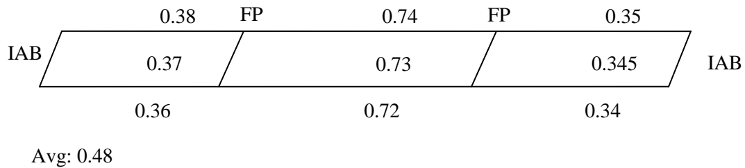
Figure 6.66. Change in length per span Bridge 2408
