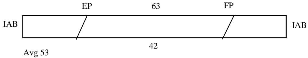
Figure 6.39. Lateral bending moment top flange Bridge 109
